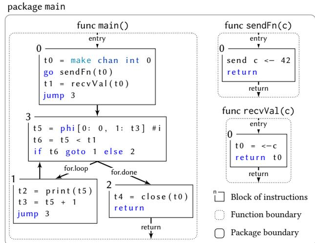
Figure 3: SSA IR built from Listing 1.
