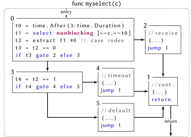
**Figure 4: Simplified SSA IR built from Listing 2.**
